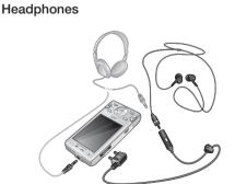
You can connect both a handsfree and headphones with a 0.14 inch (3.5 mm) plug to the phone. They can be connected to the phone at the same time.
